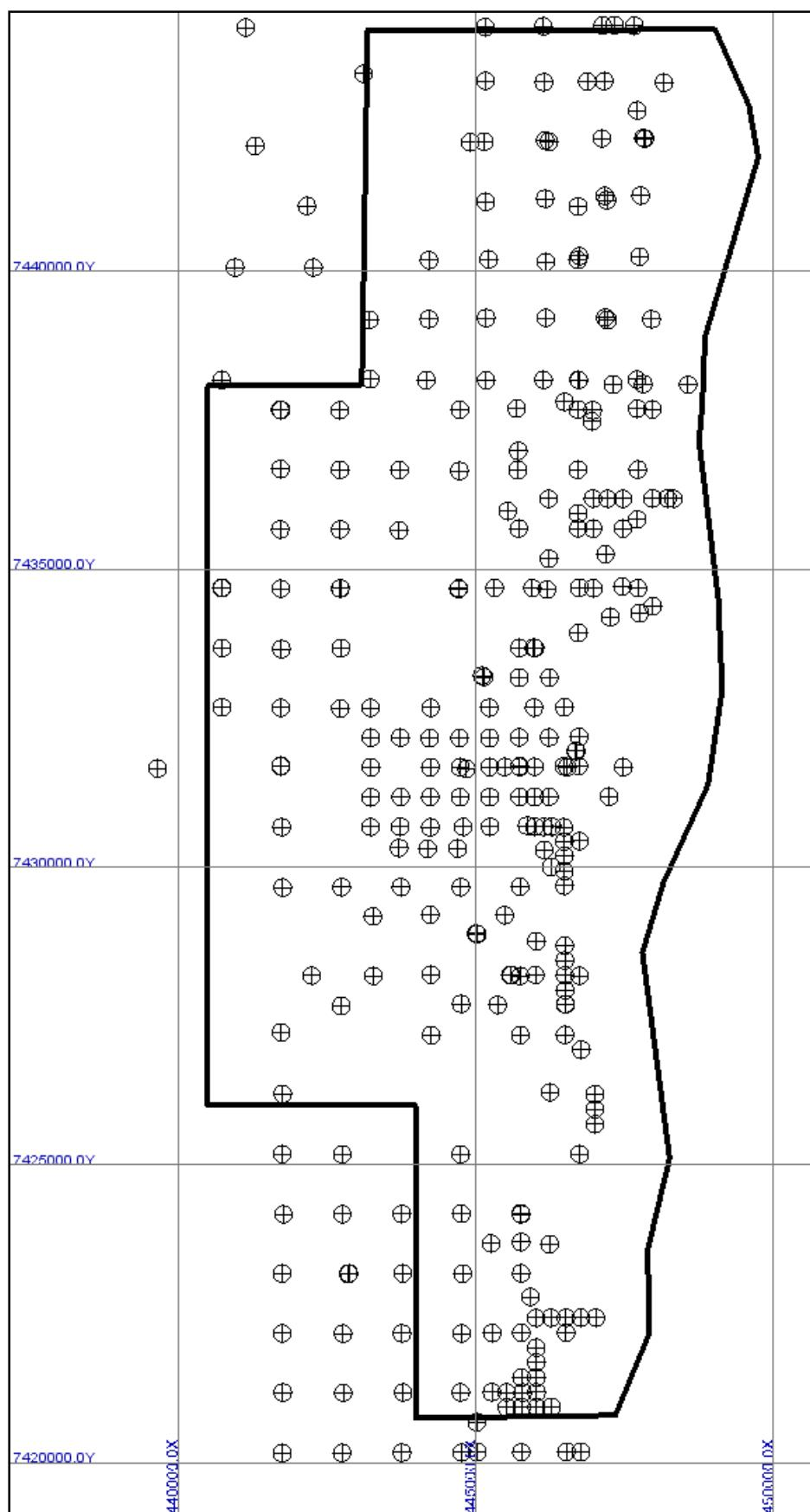
Figure 2-2: Locations of drill holes for recorded total S content for coal
