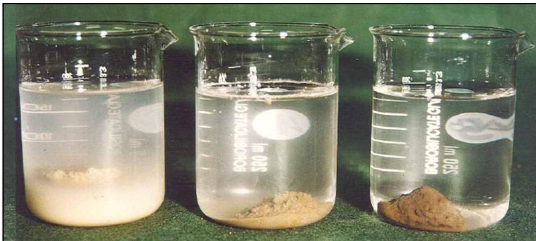
**Figure A 34: Example of Emerson tests showing highly dispersive (Class 1), slightly dispersive (Class 2 or 3) and non-dispersive (Class 4, 5 or 6) results**
